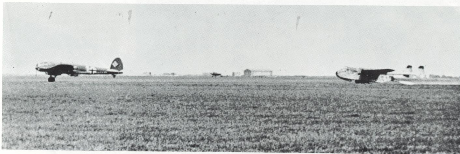
Above: A Go 242 takes off with R I-502 take-off rockets, which were ignited at the moment towing began. Below: The Go 242 has already lifted off and the HWK 109-500 A rockets have ignited.
